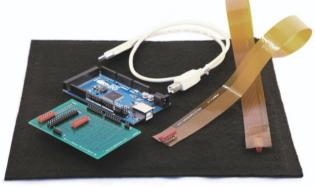
Our evaluation kits include one 12x12 or 16x16 sensor, one Arduino Mega and one shield for easy connection to the Arduino. A basic pressure map can be visualized using a Processing sketch provided free of charge.
